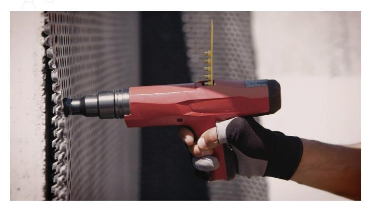
Powder-actuated tools operate like a loaded gun and should be treated with the same respect and precautions. While they are designed with safety in mind, they are potentially very dangerous and must be operated by properly trained employees who are equipped with all necessary PPE to protect against potential risks.
